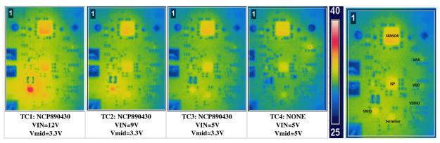
Figure 6. Thermal Images of the Reference Design Module Over Four Different Test Cases
