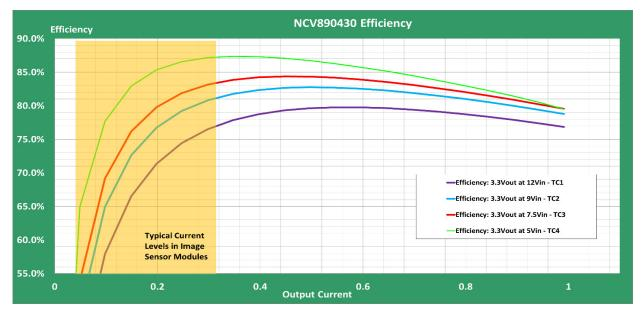
Figure 3. Efficiency Graph of the NCV890430 5–12Vin Automotive Voltage Regulator.
