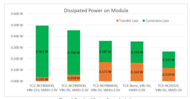
Figure 5. Results of System Power Analysis
