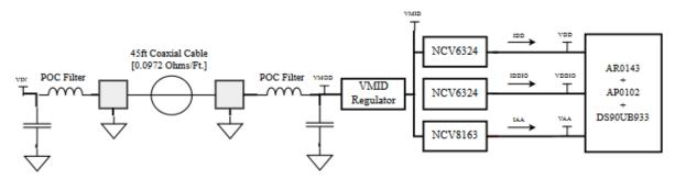
Figure 4. Diagram of the Automotive Imaging Module used to Test Design Trade-offs
